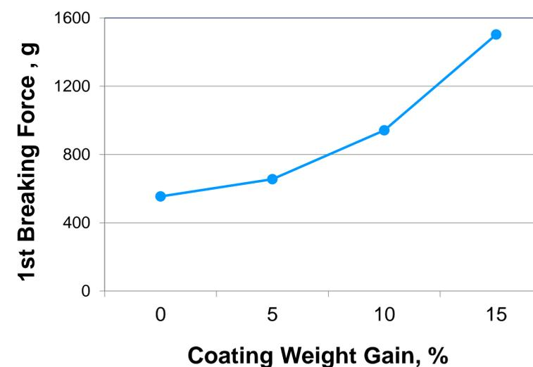
Figure 2. The effect of coating weight gain on the first breaking force of coated pellets.
