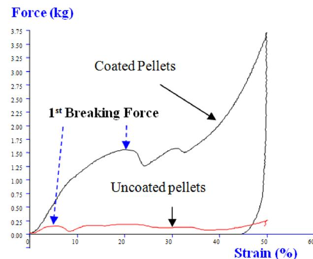
Figure 1. Force – strain curve for the pellets under compression.
